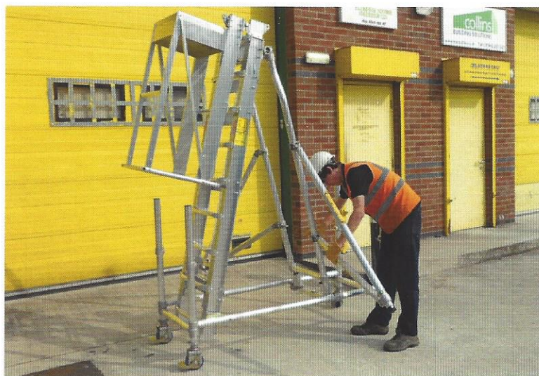
5 Position outriggers and firmly lock outrigger.
