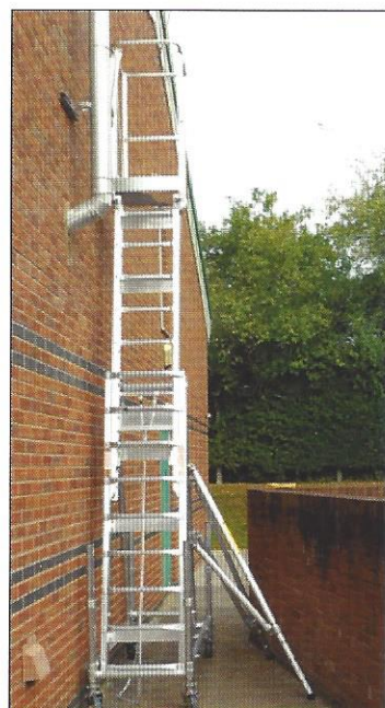
7 Insert dual drop end pins to lock pivoted top section in vertical position. Extend to height if required.
